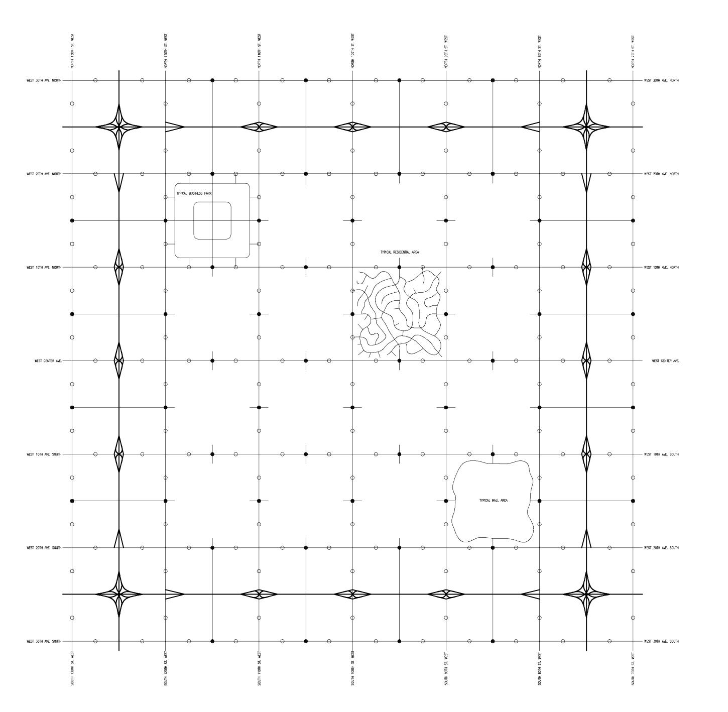
FREEWAYS ARE SPACED EVERY 10 KM (5 MI) ON A GRID PATTERN. THEY ARE ON A RIGHT-OF-WAY ADEQUATE FOR AN ULTIMATE 10 LANE FREEWAY WITH AUXILIARY LANES AND A 20 M (60 FT) DEAD ZONE OF TREES ON EACH SIDE. INTIBLLY FREEWAYS WILL BE 4 LANES WITH AUXILIARY LANES, AND EXPANDED AS NEEDED. THE EXCESS ROW ON THE EDGES WILL BE FILLED WITH TREES.
